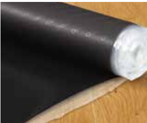
Professional SoundBloc™ PGUDLPS15, 0.95 x 15.79 m = 15 m 2 / roll PGUDLPS50, 0.95 x 52.64 m = 50 m 2 / roll The best underlay for eliminating reflected walking sound. Increases walking comfort and provides excellent impact sound insulation. Integrated vapour barrier with an overlap and tape strip included. Material: Crosslinked polyethelene foam. Thickness: 2 mm.
